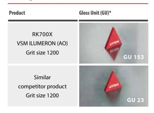
\*) The **Gloss Unit (GU)** of is the measuring unit of a gloss metre. 0 GU stands for a perfect matt finish. High-gloss surfaces have a typical GU value of 70.
